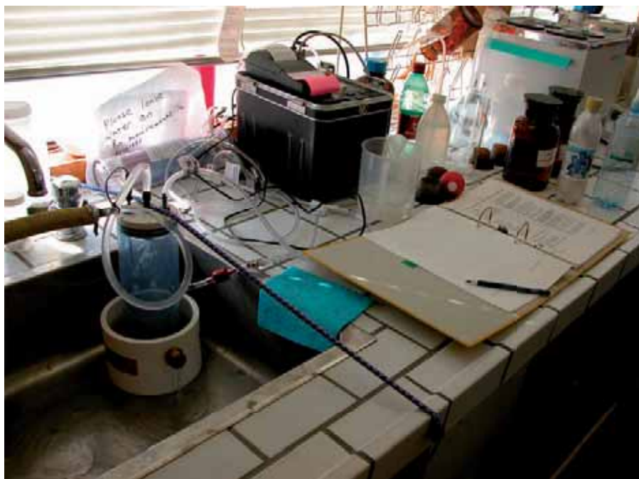
FIG. III-4. Photo of the RAD-7 radon detector (small dark box with printer on top) and RAD AQUA system (blue cylinder) in operation on board the Joint Danube Survey ship Argus in 2007. River water is being pumped through the RAD AQUA where it releases radon gas that is then pumped into the RAD-7 for detection of radon-222.
