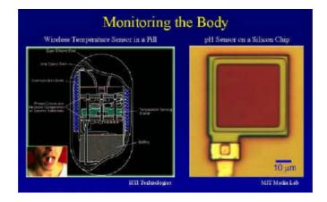
**Figure 2.** New generation of wearable sensors enable real-time wireless readout of internal bodily signals such as temperature or pH.
